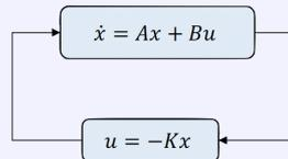
To stabilize the system using full-state feedback, we must be able to access all of the system's states. Unfortunately, this is not always possible.
