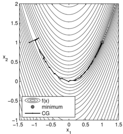
Solution path of the steepest descent and conjugate gradient methods
