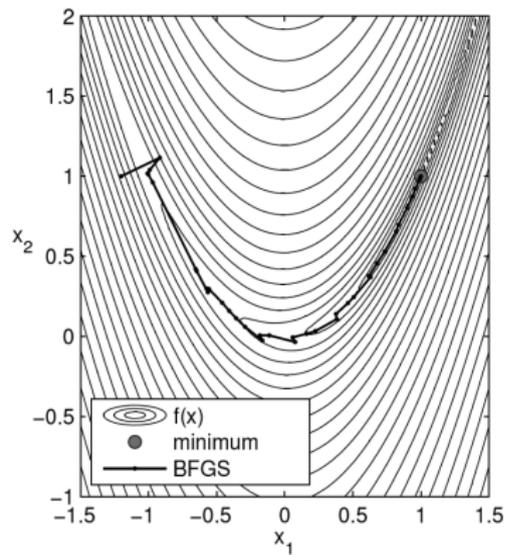
Solution path of the modified Newton and BFGS methods
