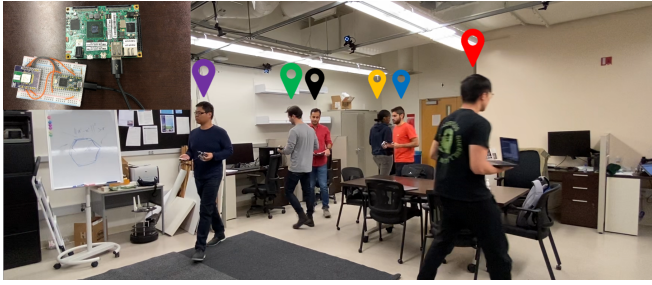
Fig. 5 – The first experiment was performed by 6 pedestrians, each carrying an UWB transceiver (left-top).
