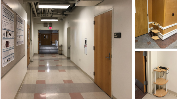
Fig. 4: The experiment setup in the Engineering Gateway Building at UCI campus. The small plots in the right show beacons B2 and B3 that are located in the corners. As we can anticipate from our beacon locations, as the pedestrian walks along the reference trajectory, the collected range measurements with respect to the beacons will vary between LoS and NLoS conditions.
